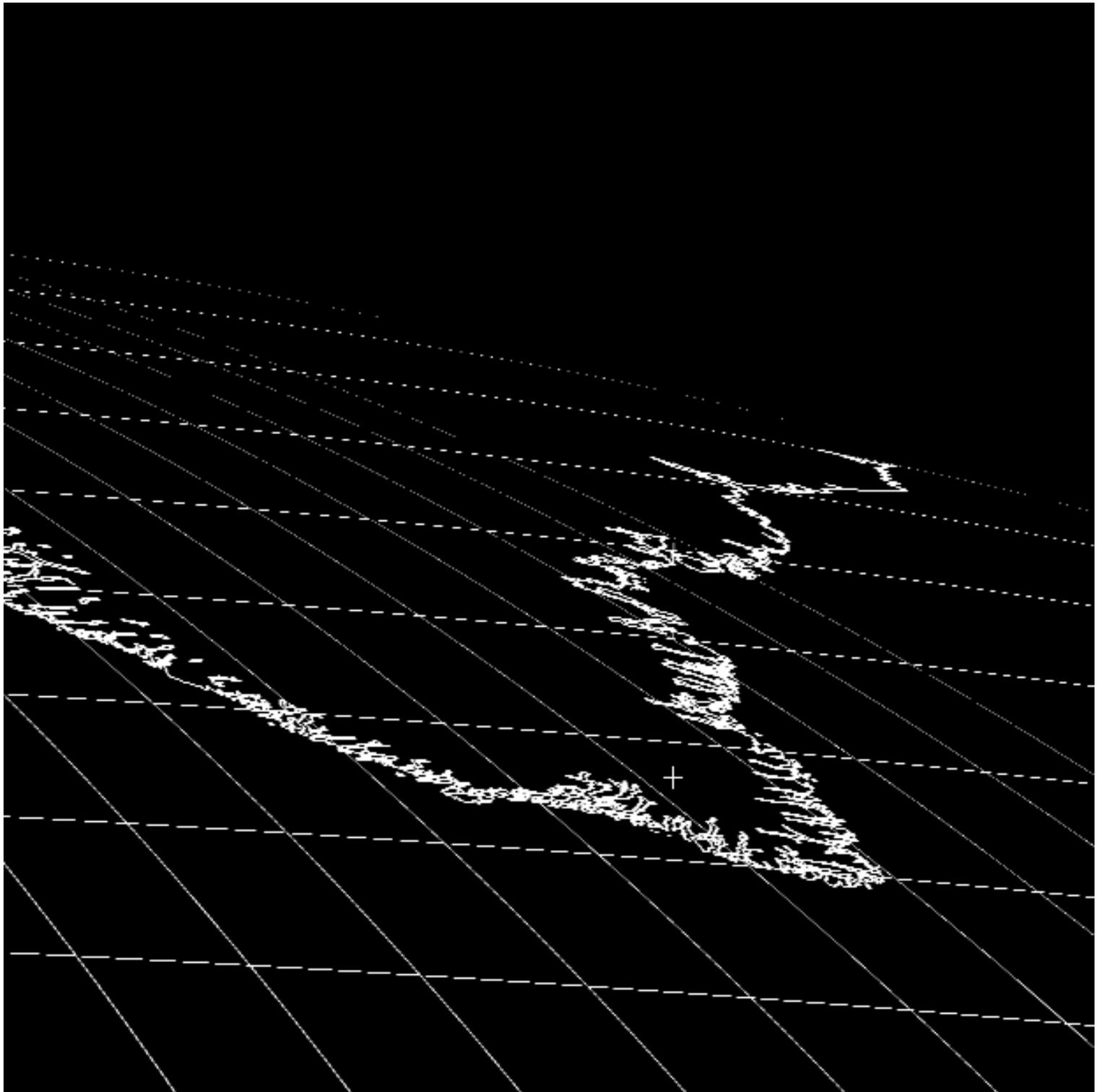
The "+" marks the reported impact point at 61.4N, 44.4W. Latitude and longitude lines are sketched at 2 degree intervals, based on the reported GOES earth-navigation. At this time, the navigated map's coastlines fall 3 pixels south and one pixel west of the observed coastlines, within the GOES earth-navigation error tolerances of 4 visible pixels.
